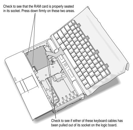
Make sure the keyboard cables are still properly connected.
